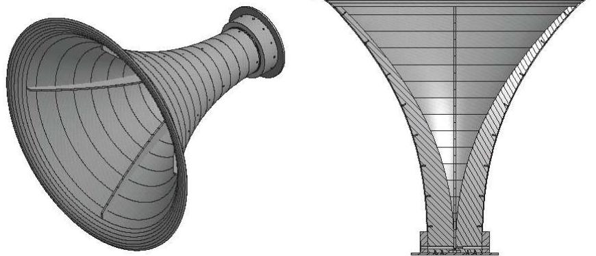
Figure 4.11: Three-dimensional CAD drawings of the high-gain quad-ridge horn. Feed diameter is 82 cm ( $1.9\lambda_{lo}$ ) and length is 73.2 cm ( $1.7\lambda_{lo}$ ) with  $f_{lo} = 0.7$  GHz
