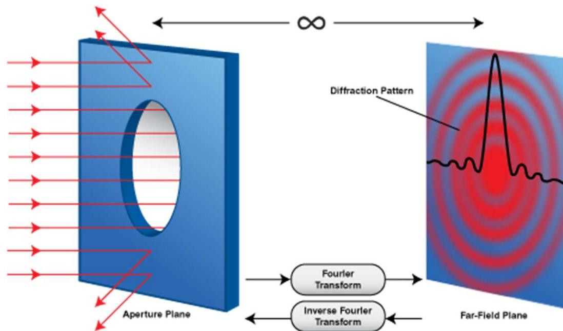
Far-field beam pattern is Fourier transform of aperture plane electric field distribution
