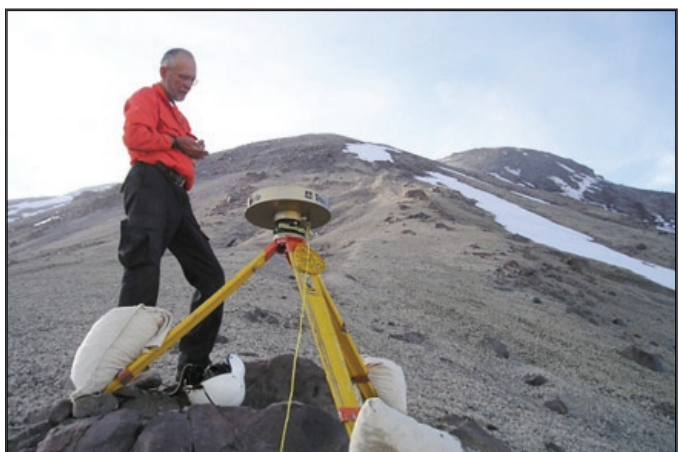
Scientist collecting information from a Global Positioning System (GPS) station on Mount St. Helens. USGS
