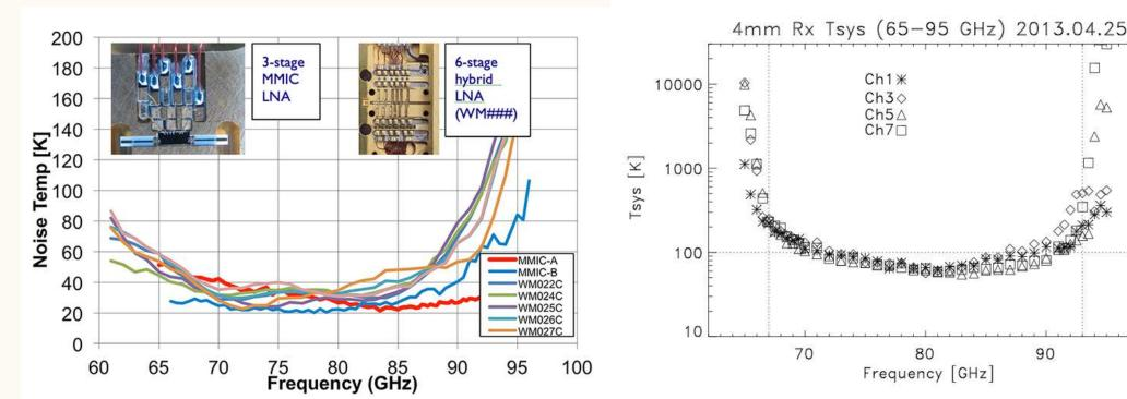
(Left) The performance of different cold amplifier designs measured in the lab. (Right) Recent system temperature measurements on the sky as a function of frequency for each of the 4 channels (2 polarizations and 2 beams, "ch1,3,5,7") shown as symbols for the new amplifiers.
