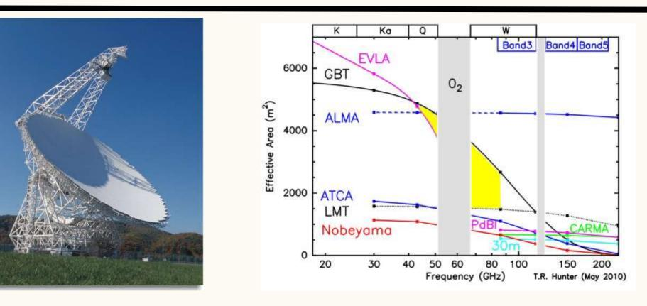
The GBT has the largest effective collecting area of any telescope on earth operating from 40 –84 GHz (shown in yellow). The GBT is sensitive to extended emission unlike interferometers and can provide important shortspacing data for many VLA and ALMA programs
