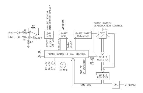
Figure 5: Detector readout for one frequency channel.
