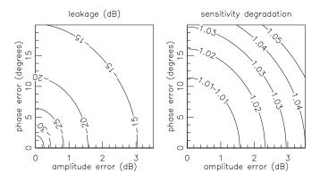
Figure 2: Leakage and sensitivity degradation due to differential passband errors between the two arms of the radiometer, in total power mode.
