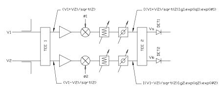
Figure 1: Differential radiometer.
