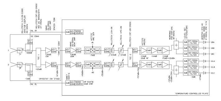
Figure 4: Radiometer front end. This diagram shows the details for just one polarization (horn1Right-horn2Left). The circuit for the other polarization is identical.
