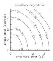
Figure 3: Sensitivity degradation due to differential passband errors between the two arms of the radiometer, in phase switched differential mode.
