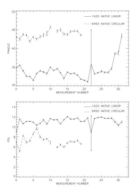
Crosscorrelation (9493 MHz) gives better results than differencing (1420 MHz) for position angle measurements. You NEVER see wild fluctuations with crosscorrelation, while they are common with differencing. (At 1420 MHz 3C286 is  $\sim 1.5T_{sys}$ ; at 9493 MHz 3C286 is  $\sim 0.5T_{sys}$ ). (POL for 9493 MHz is displaced downward by 4 for clarity).
