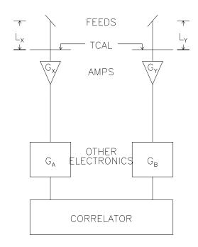
Cable lengths introduce phase delays. Cables are never identical!
