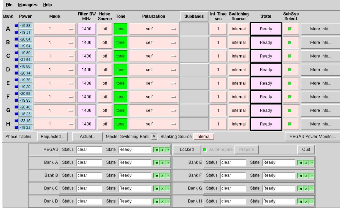
Figure 9.4: The VEGAS CLEO window with all 16 beams connected to Argus. The VEGAS power levels should be \sim -20 \pm 3 dBm when balancing on blank sky. When observing the vane, the associated levels would be \sim -15 dBm since the ambient vane temperature is \sim 3 times the typical sky level. In this example, VEGAS Bank H1 which is connected to Argus beam-6 is not in range.
