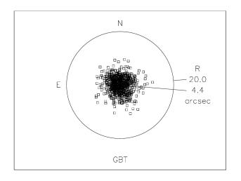
**Figure 5.** Pointing performance of the MVET'ed pointing model on the 2017-2018 dataset, with offsets fit to each session (this simulates all-sky relative pointing performance).
