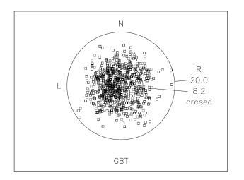
**Figure 4.** Pointing performance of the MVET'ed pointing model on the 2017-2018 dataset, given fixed offsets (this simulates blind pointing performance).
