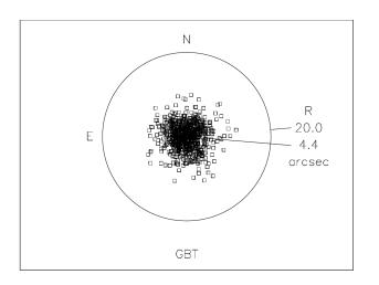
**Figure 2.** Pointing performance of the GBT's standard (5s) pointing model on the 2017-2018 dataset, with offsets fit to each session (this simulates all-sky relative pointing performance).
