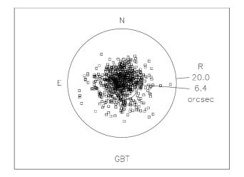
**Figure 1.** Pointing performance of the GBT's standard (5s) pointing model on the 2017-2018 dataset, given fixed offsets (this simulates blind pointing performance).
