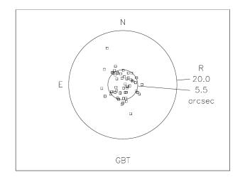
**Figure 3.** Pointing performance of the GBT's standard (5s) pointing model on the 2021 dataset, with CAL and IE offsets fit to the session (this simulates all-sky relative pointing performance).
