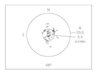
**Figure 6.** Pointing performance of the MVET'ed pointing model on the 2021 dataset, with CAL and IE offsets fit to the session (this simulates all-sky relative pointing performance).
