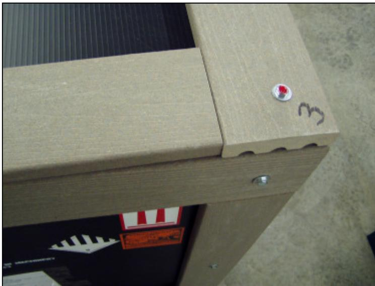
2. Using the 14mm wrench, remove the larger red bolts at the bottom of all 4 sides.
