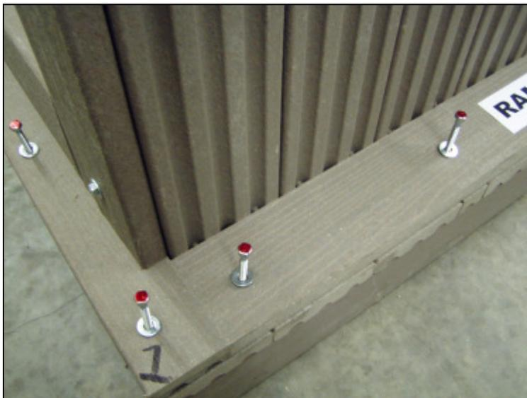
3. Remove the remaining red bolts on the sides next to the “RAMP” end. Next, remove the end marked “RAMP” off of the maser crate.
