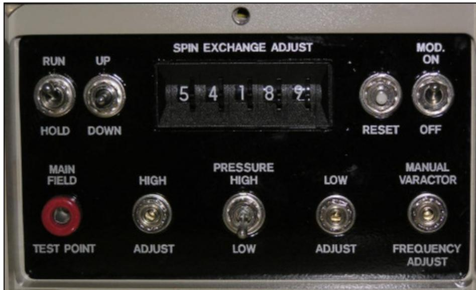
After the register has been reset, the maser will automatically return to its tuned position in a few days. The register must be reset before it will automatically tune. Refer to the maser manual (see Section 3 on the Cavity Servo System of the Operating Manual, #75666-201) for a more detailed explanation.
