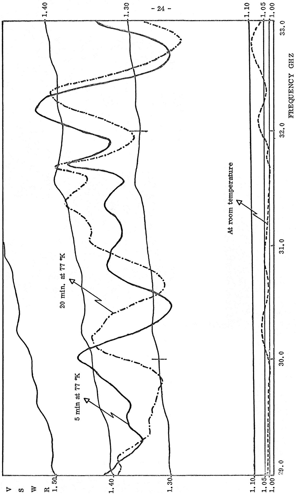
FIG. 14 - VSWR OF LABORATORY ASSEMBLED LIQUID NITROGEN LOAD
