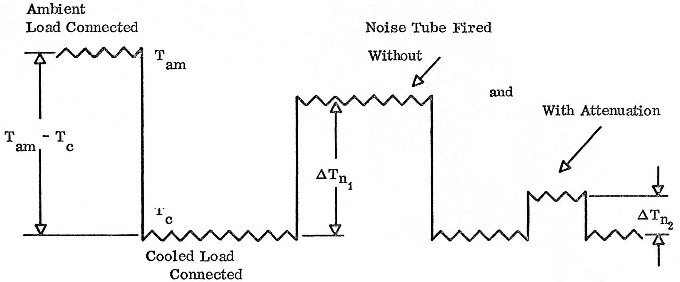
FIG. 2 -- TYPICAL CALIBRATION CHART (NOT TO SCALE)
