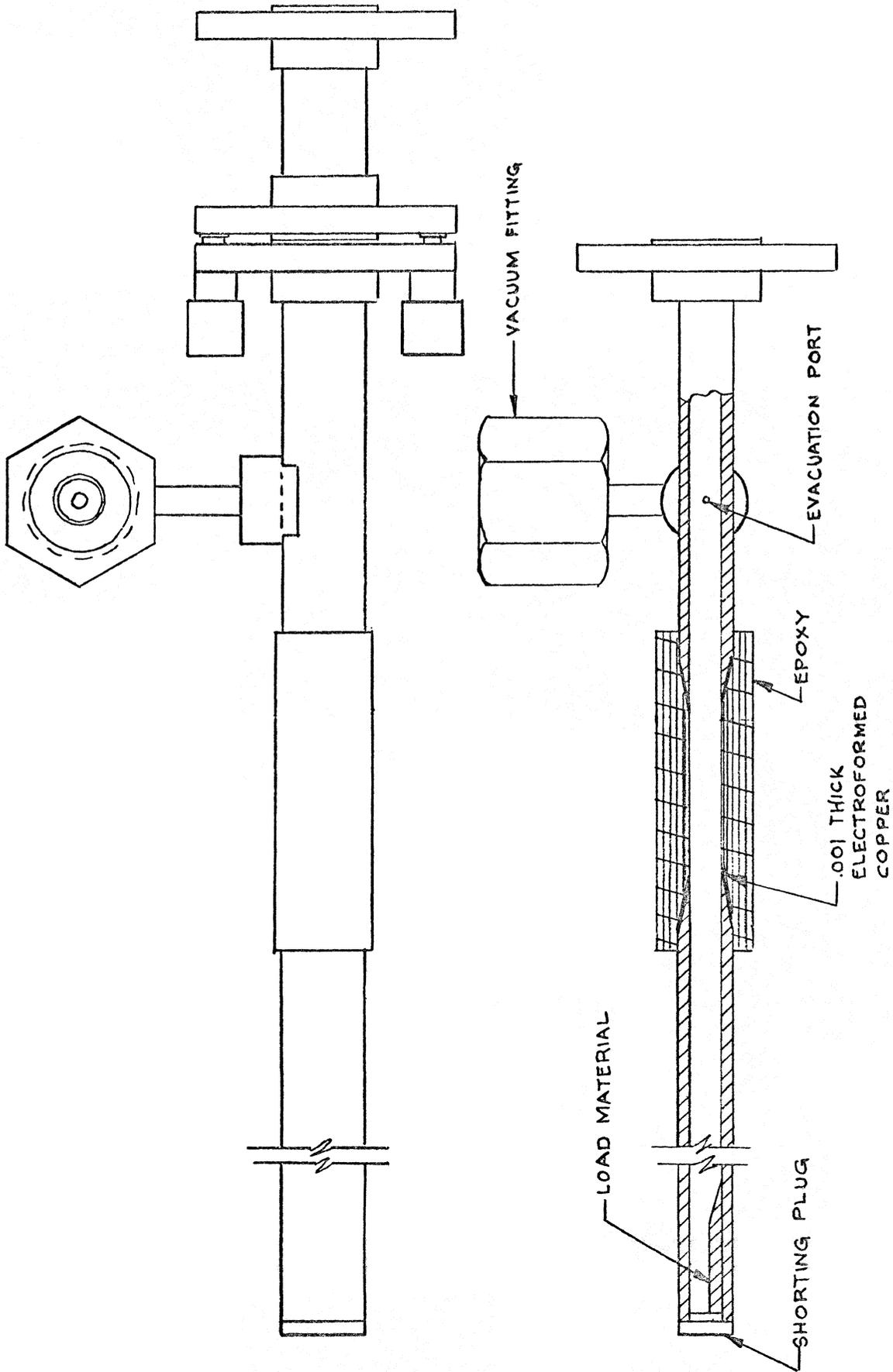
FIG. 5 - WAVEGUIDE LOAD WITH THERMAL ISOLATION SECTION
