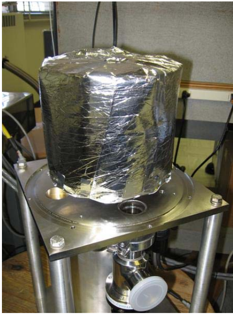
Figure 11: A cylindrical heat shield wrapped in superinsulation added to the cold finger.
