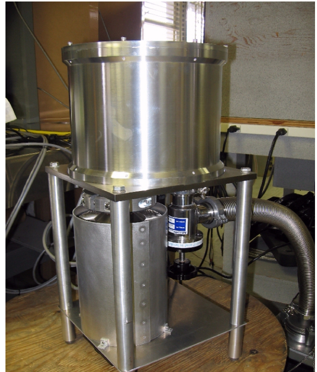
Figure 4: An air shroud installed around the refrigerator case and fins. A 100cfm fan is located below the shroud, pulling air downward.
