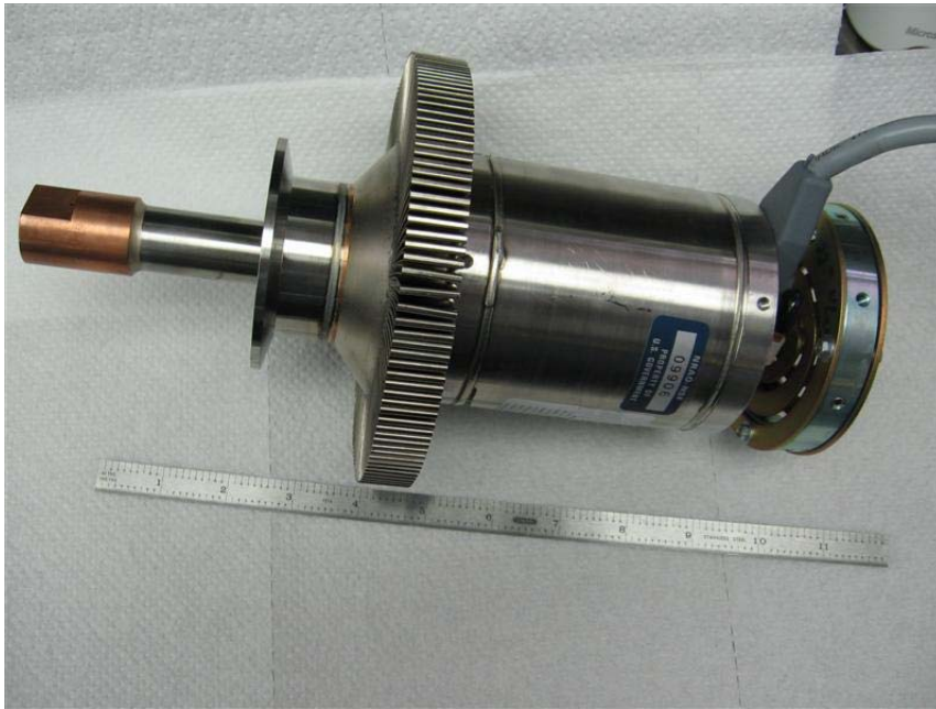
Figure 2: The GT cryocooler. The cold finger is to the left and the vibration damper is to the right. The unit weighs 8 lb., 14 oz.
