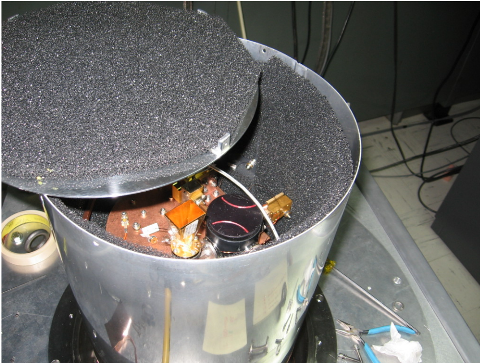
Figure 15: Absorber lining the radiation shield.
