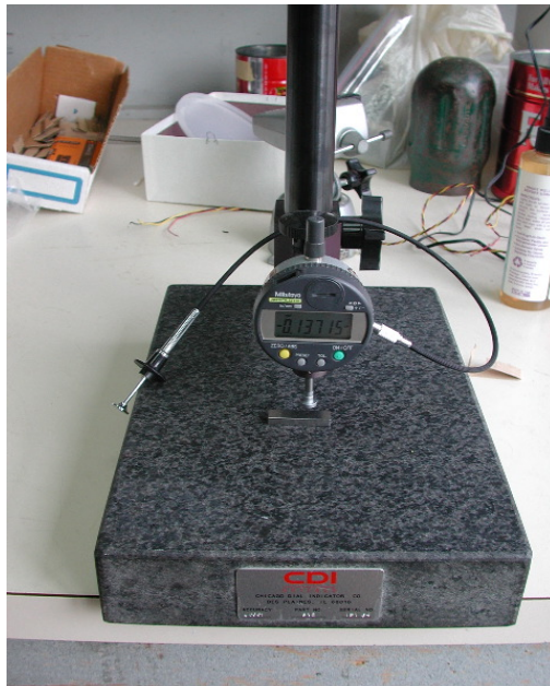
Digital micrometer and granite plate
