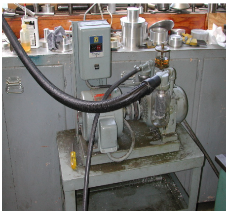
GAST vacuum pump (Small hose is vacuum line, large hose is exhaust)
