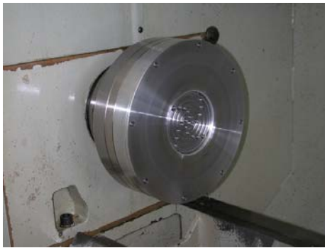
Mounted lathe vacuum chuck
