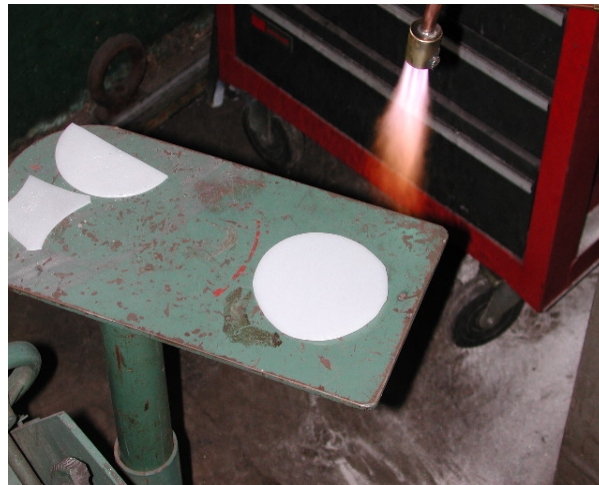
Ready to pass the oxidizing flame over the HDPE
