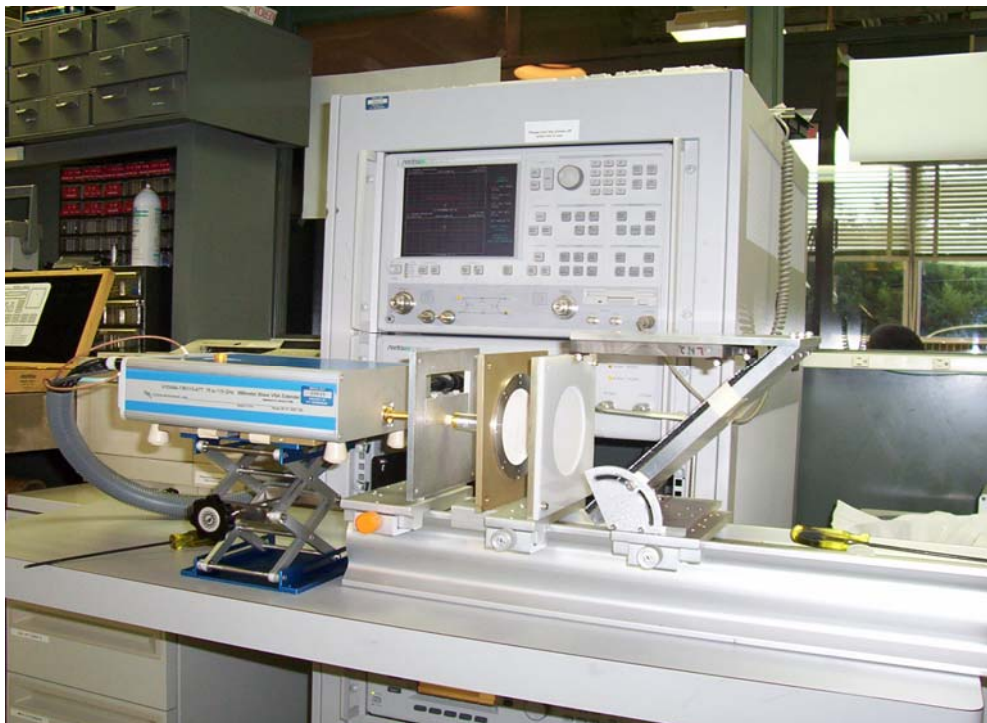
Anritsu VNA, Oleson WR10 extender, feedhorn, IR filter, quartz window, load
