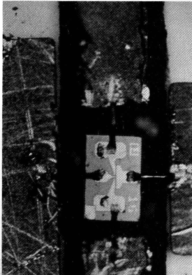
Fig. 2.11. Microscope photograph of stage three HEMT. For size reference the chip is .008" long (left to right in photo) by .012" wide. The bond wires are .7 mil diameter gold bonded at 105C stage temperature. The chip is attached with Epotek H20E epoxy.
