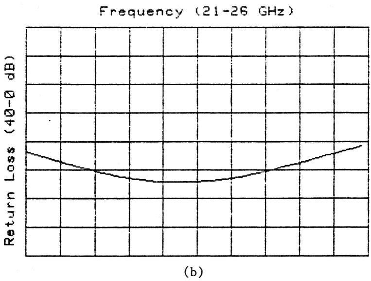
Fig. 4. Theoretical return loss of d.c. block with  $L = .054''$  and (a)  $w/h = s/h = .12$  and (b)  $w/h = s/h = .14$  calculated by "dcblocka".
