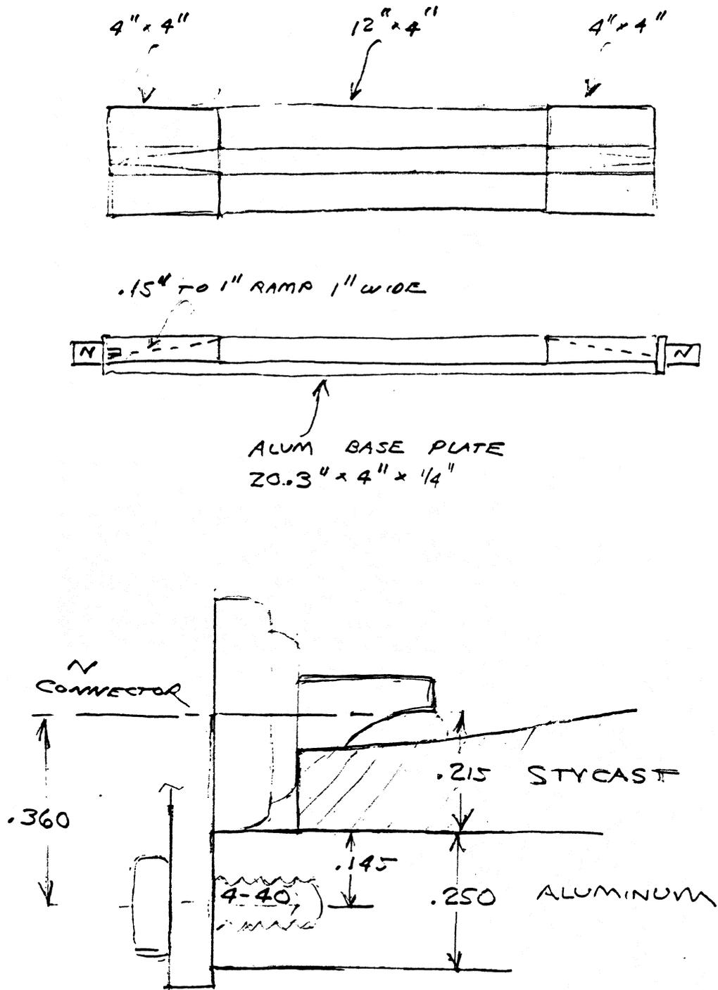
Fig. 5. Test fixture for scale-model measurements.
