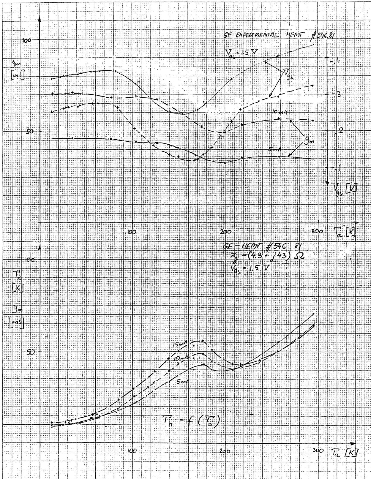
Fig. 16. The cooling curves for 8.4 GHz, single-stage GE HEMT amplifier with the source impedance optimal for cryogenic noise performance.
