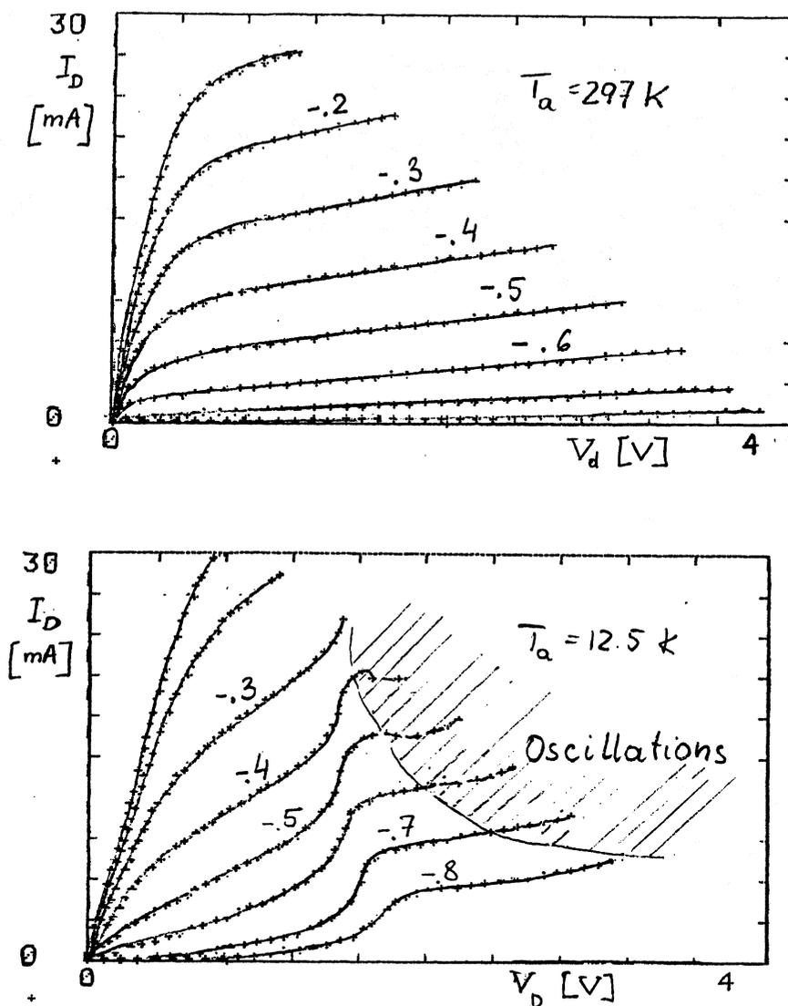
Fig. 7. The drain characteristics of NE71083 (32-4) FET at  $297\text{K}$  and  $12.5\text{K}$ .
