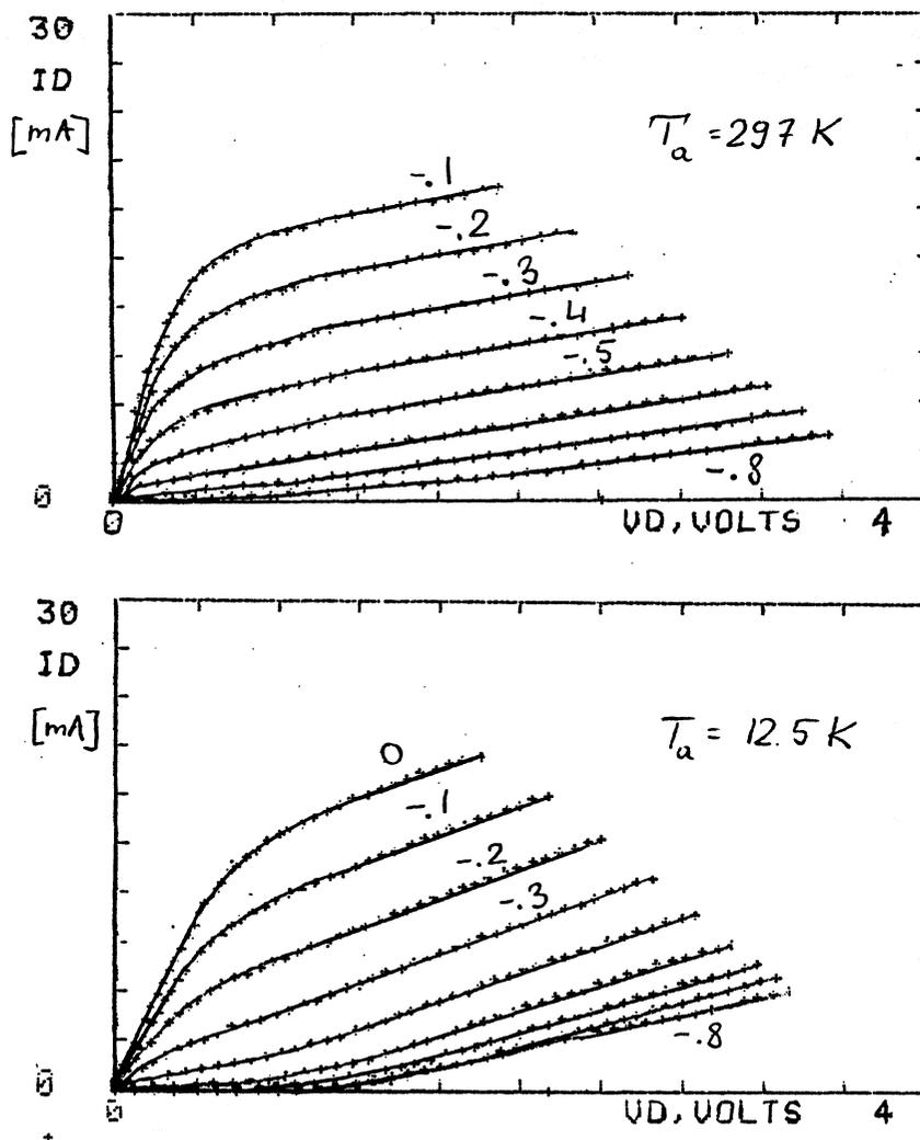
Fig. 10. The drain characteristic of the 2SK575 (YY925) FET at 297K and 12.5K.
