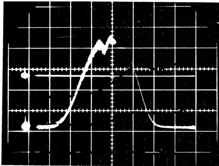
Figure 10 1400 Mc -- entire system (front end and back end), switch locked in signal; gain modulator locked in comparison; bandpass 1416 Mc to 1423 Mc; centered on 1420 Mc.
