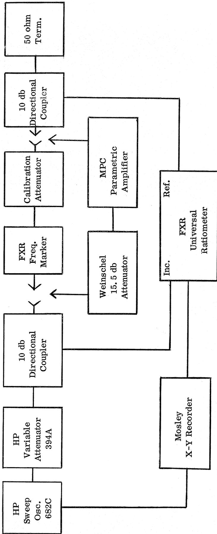
Figure 7. Test equipment arrangement to plot the gain-bandpass characteristics of the parametric amplifier. The variable attenuator was set at 26 db. This was the maximum allowable attenuation for proper operation of the ratiometer. Results of this test were unsatisfactory due to saturation of the parametric amplifier. Refer to Figure 8 for overload characteristics and results of this test.
