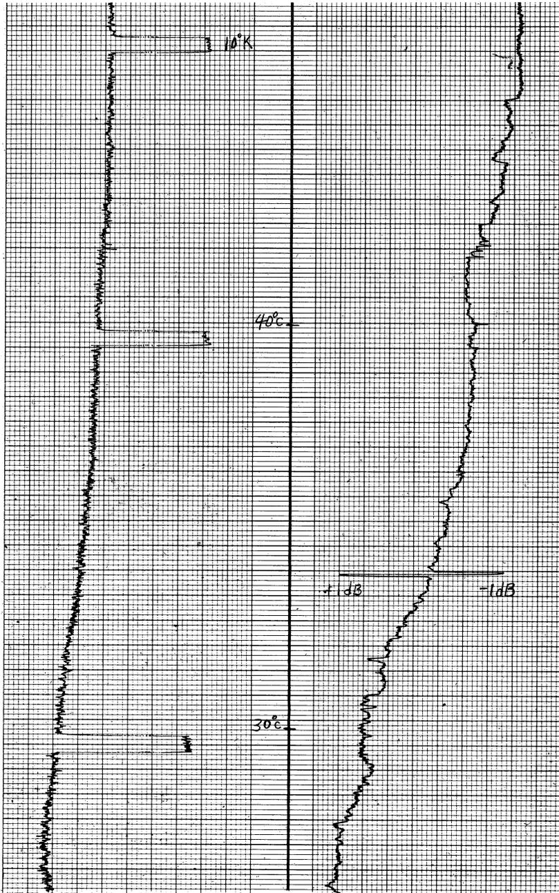
Figure 11. Ambient temperature vs. output.
