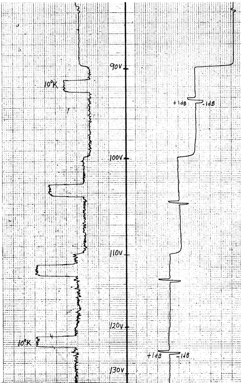
**Figure 13. AC Line Voltage vs. Output**
