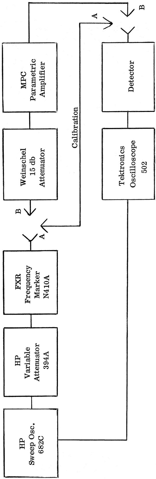
Figure 1. Test equipment arrangement used to observe gain-bandpass characteristics and for making adjustments on the parametric amplifier. The variable attenuator was set at 50 db. Scope sensitivity  $200 \mu\text{V}/\text{cm}$  with 3 cm vertical deflection.
