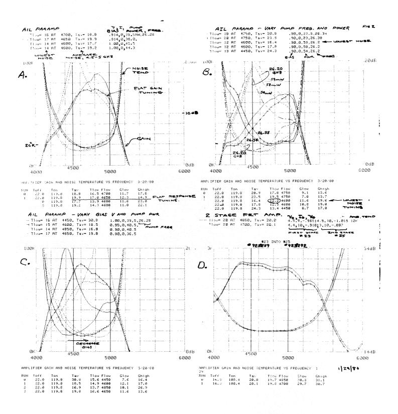
Figure 2 - Gain and noise performance of AIL paramp and NRAO 2-stage GASFET amplifier.
