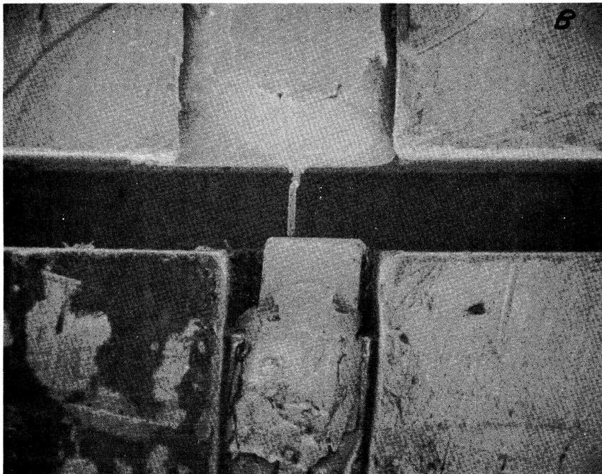
Fig. 6. Electron microscope photographs of the 2-mm mixer mounts: top is mixer A; bottom is mixer B.
