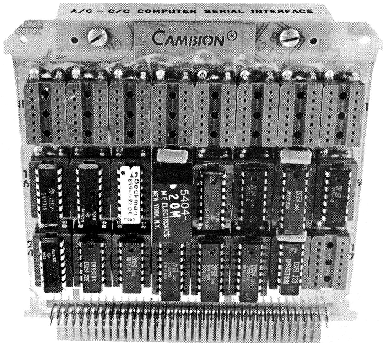
A small Cambion circuit card installed in the DDP-116 computer provides the serial interface to the digital delay system. A 20 MHz  $\div$  16 clock provides an asynchronous data rate of 1.25 M bits/sec. The circuit schematic (next page) shows the signals that connect to the computer and delay system.
