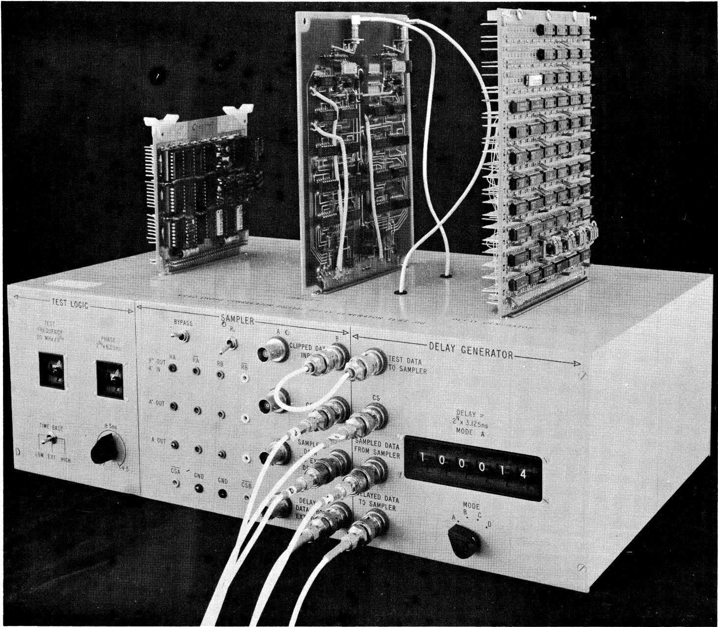
The test set will completely test the sampler card and the delay generator card by manipulation of the controls which are self explanatory. The phase control on the left adjusts the phase between the test waveform and the sampler clock.
