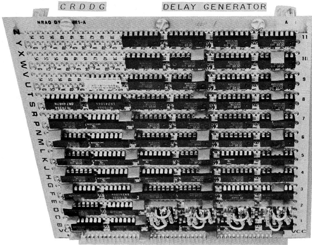
The pix of the delay generator shows the "fine delay system LC delay lines at the bottom right corner. The card is a "standard" large Shalloway wire wrap card which holds 66 IC's when laid out as 16 pin chips using the "card shark" wire wrap program. Four of these cards are required in the system as shown in the previous functional block diagram.
