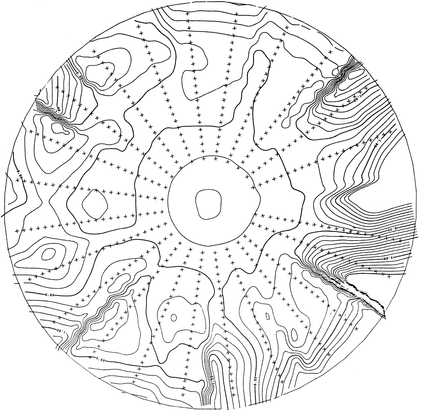
Figure 8 — (a) and (b) — Maps of the departures of the reflector surface from the best-fit paraboloid. (a) and (b) are derived from separate sets of measurements. Contour interval = 0.2 mm.
