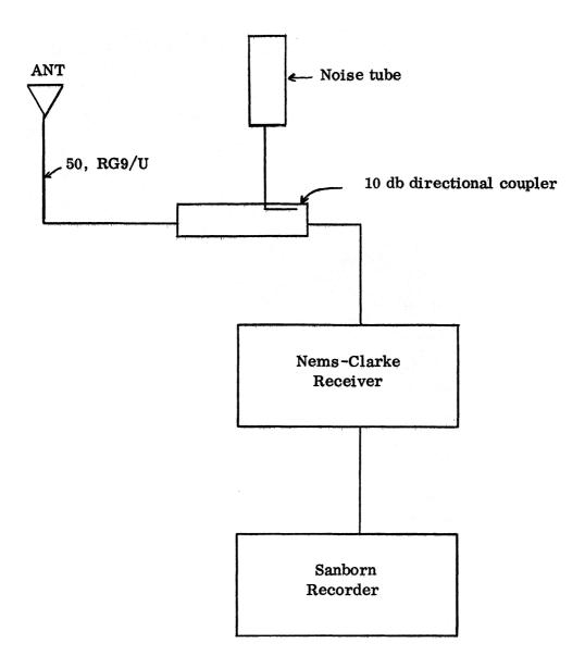
BLOCK DIAGRAM - TEST SET-UP
