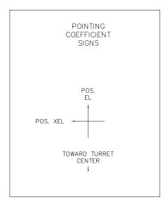
Figure 1: Diagram showing the signs of the beam offset coefficients versus feed displacements. The view is again looking down on the turret with the top toward the main reflector and the bottom toward the turret center.
