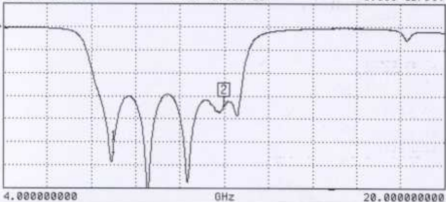
S11 FORWARD REFLECTION LOG MAGNITUDE REF=0.000 dB 5.000 dB/DIV
