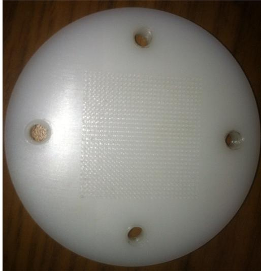
Figure 2.8: The *Argus* window, which is made from 0.5" thick ultra-high-molecular-weight polyethylene.
