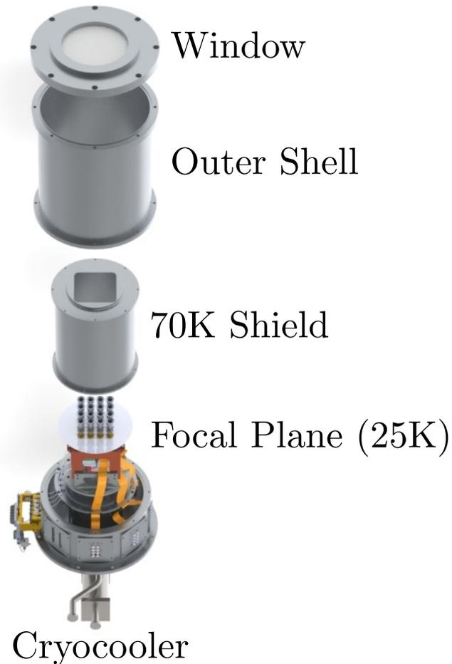
Figure 2.13: A CAD drawing of the *Argus* cryostat. The connector feedthroughs are installed on the octagonal base. The cylindrical outer shell and the 70 K heat shield can be removed for full access to the focal plane array. The circular plate at the top of the drawing that holds the window was used for lab testing and was later replaced by a larger plate that adapts to the 24" diameter holes in the GBT turret.
