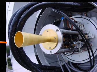
Holography Receiver at top of secondary
