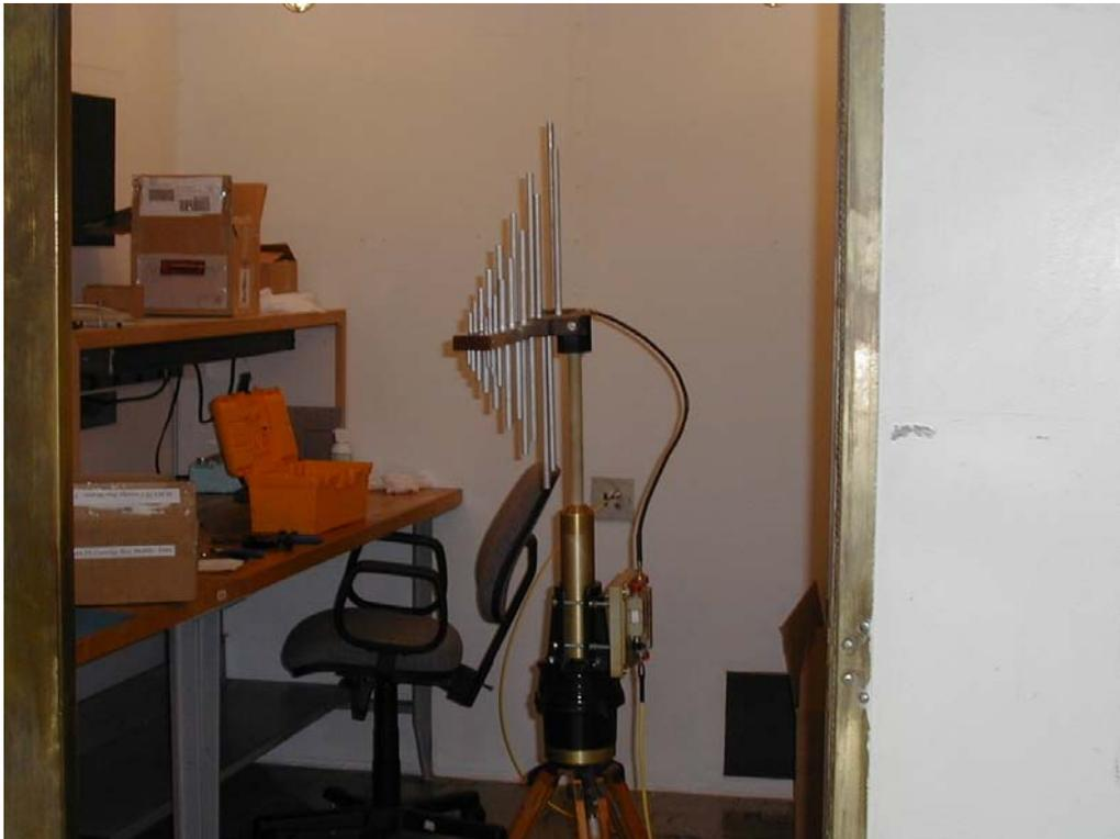
Figure 2: Log Periodic Antenna in Shielded Room
