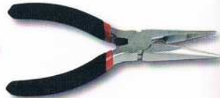
Long-nosed pliers are needed to bend the leads on components and hold wires or other parts while you solder.
