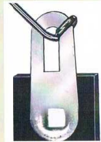
Attach the wire to a soldering terminal or soldering lug.
