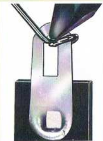
Heat the wire and the lug.
