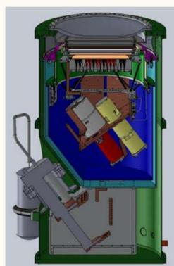
Mustang is a 3mm bolometer camera for the GBT. The detectors for Mustang-1.5 are 3-8x more sensitive than the current Mustang. Mustang-1.5 (available 2013) will provide similar mapping speeds to ALMA, while Mustang-2 with 332 detectors will map more than 10x faster than ALMA.
