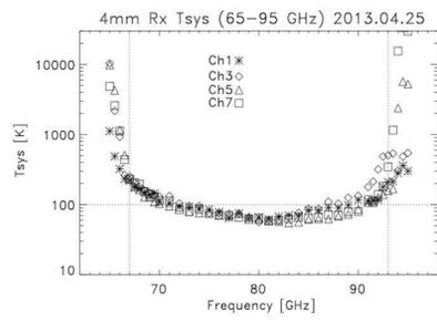
(Left) The performance of different cold amplifier designs measured in the lab. (Right) Recent system temperature measurements on the sky as a function of frequency for each of the 4 channels (2 polarizations and 2 beams, "ch1,3,5,7") shown as symbols for the new amplifiers.
