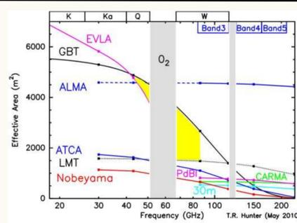
The GBT has the largest effective collecting area of any telescope on earth operating from 40-84 GHz (shown in yellow). The GBT is sensitive to extended emission unlike interferometers and can provide important short-spacing data for many VLA and ALMA programs
