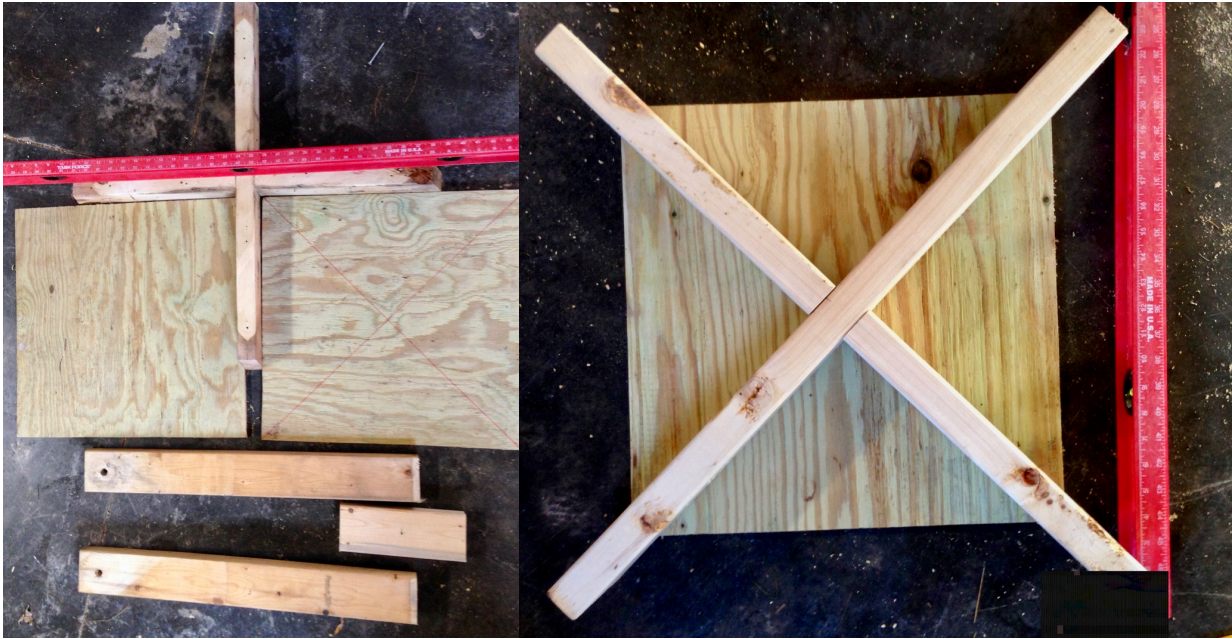
Figure 6: Assembly of the cross pieces to make the base legs. The image at left shows how the plywood base and protractor are used to square the base legs. At right, the base is shown attached to the legs.
