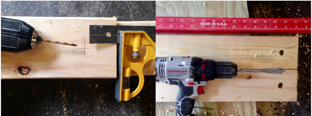
Figure 7: Drill holes in vertical pieces for Elevation Tilt. The left image shows measurements 1 3/4-inches from all edges of the one of the 27-inch long vertical forks. The image on the right shows 5/8 inch holes drilled in both fork pieces with the spade drill bit.
