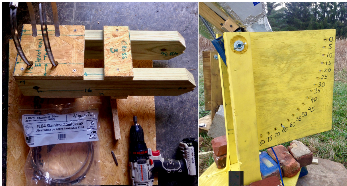
Figure 17: Completed elevation shelf and final base, painted and numbered. At left the complete elevation shelf is shown with two large (7 inch diameter) stainless steel clamps for attaching the horn to the base. At right, the elevation shelf is attached via a 1/2 inch diameter threaded bar, 12 inches long. Use two washers and two wing nuts to hold the elevation axis in place. Paint and then number the elevation angles for each slot.
