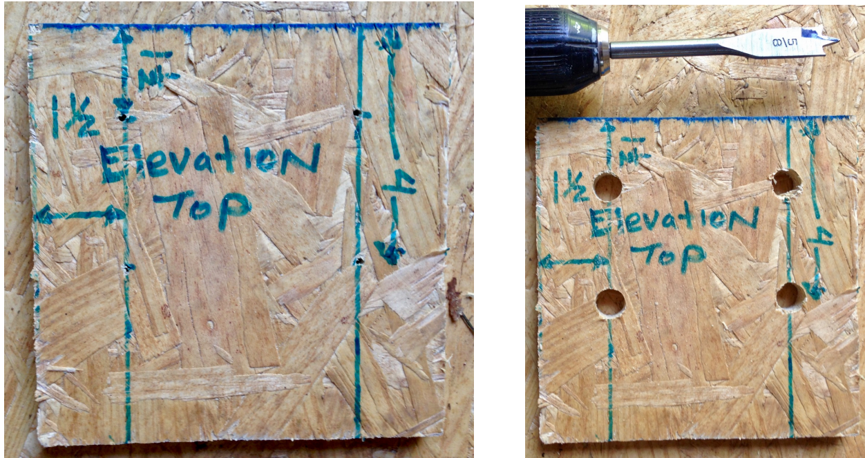
Figure 14: Drilling holes in Elevation top for Attaching horn. The elevation shelf top has 4 holes for clamping the horn to the tilt shelf. First measure 1 1/2-inch and draw lines 1 1/2-inches from the edge of the two sides. Then with the 1/8-inch drill bit, pre-drill holes 1 1/2 and 4-inches from the front of the top base, as is shown on the left. Then use the 5/8-inch spade drill bit to make holes wide enough for the metal clamps, as shown on the right
