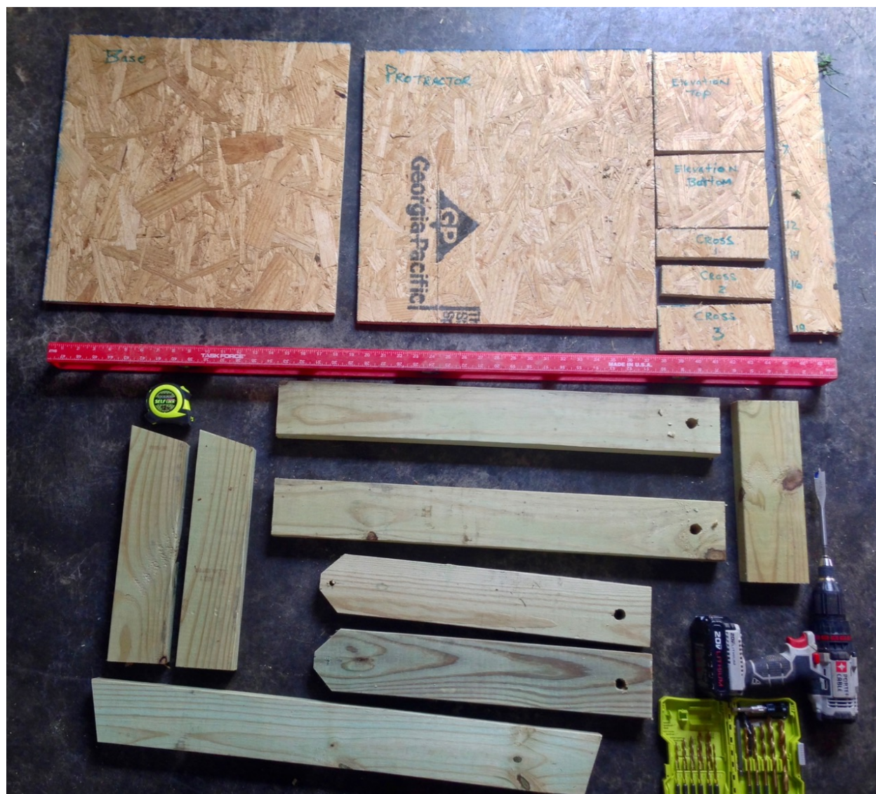
Figure 2: Wood parts of Science Aficionado Telescopes, before assembly. The pieces cut from a 48-by-19-inch plywood sheet are above the 4-foot long re ruler.. Below the red ruler are pieces cut from two 2x4s. Some of the tools are also shown, including tape measure, set of drill bits and electric drill..
