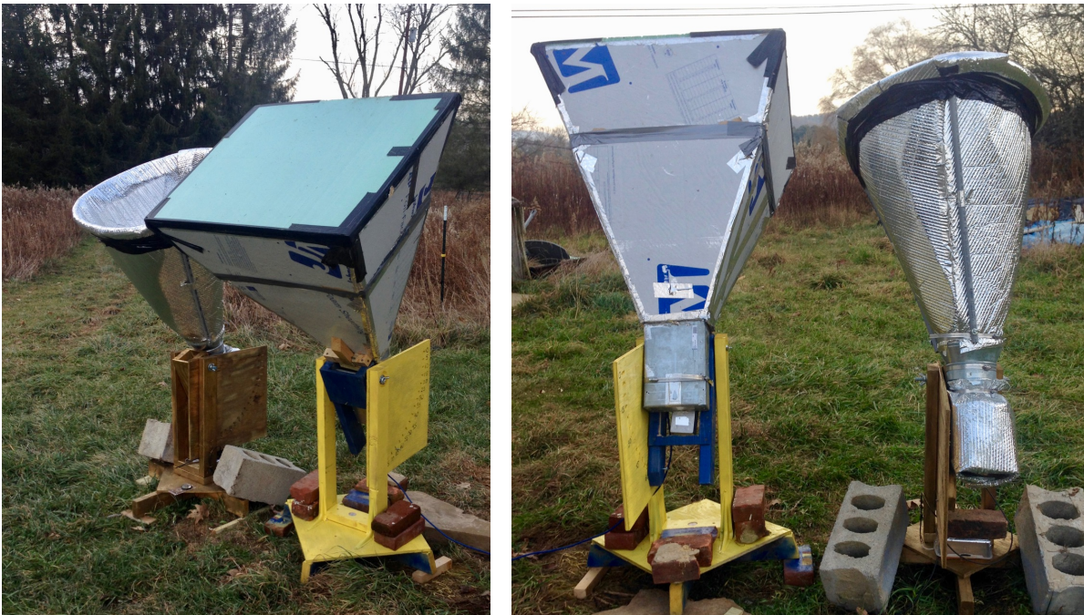
Figure 1: Two Science Aficionado Telescopes. At left, the front of two telescopes is shown. One telescope is constructed out of reflective foam sheets and the other is made of bubble wrap, held in shape by segments of conduit. At right, the rear of these two telescopes is shown. The telescopes can stand by themselves if there is no high wind. Because these telescopes were left outside, the base is weighed down with concrete blocks and bricks.
