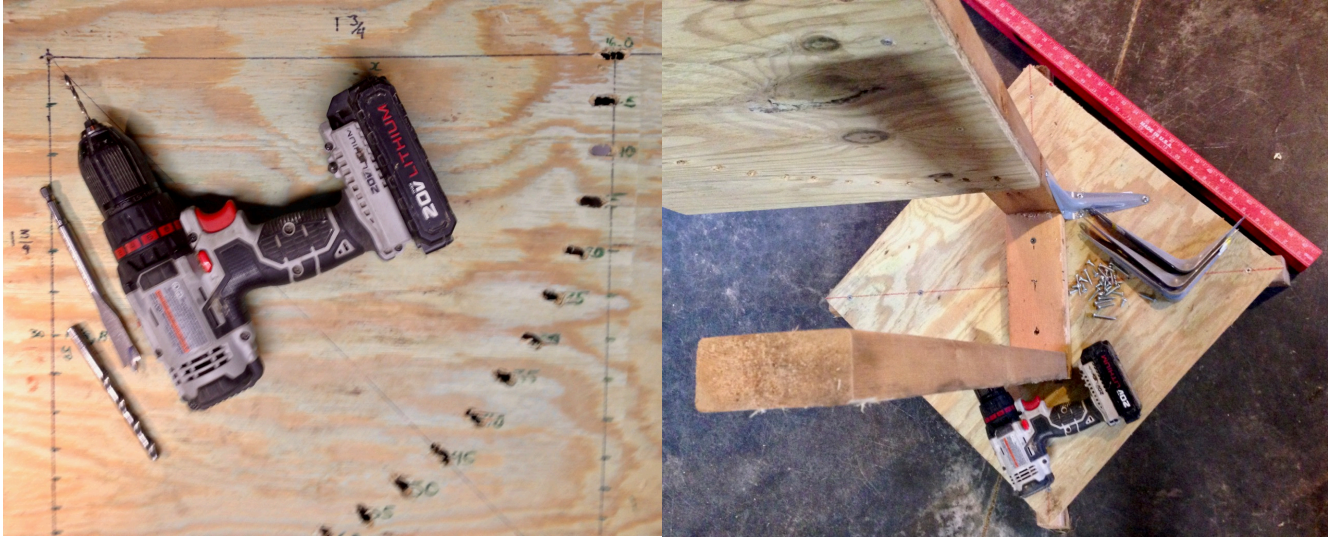
Figure 12: Drilling the protractor slots. At left the image shows the protractor slots re-drilled with a 1/4 inch drill bit. First drill where you've previously drilled the 1/8 inch pilot holes. The slide the 5/16 inch drill bit between the two holes make a slot about 1/2 inch long. The slot is needed to account for any inaccuracy of assembly of the base board. At right the assembled vertical forks with protractor install in-between the two forks.
