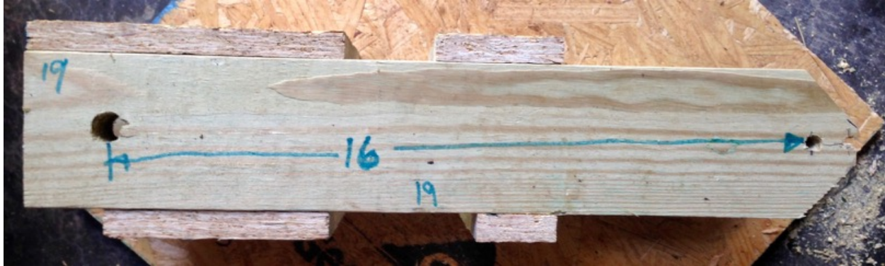
Figure 16: Side view of the Elevation Tilt Shelf for Attaching horn. One bottom part is the 5 inch wide cross piece, aligned with the two elevation axis holes. The other bottom part is a 2-inch wide cross piece, 12 inches back from the front of the shelf. Attach these pieces with 1 1/2-inch screws
