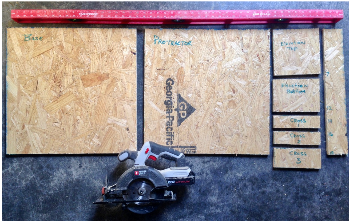
Figure 4: All plywood parts cut. The telescope base and protractors are exactly the same size, 19-inches square. The smaller parts are for the elevation tilt part of the base.
