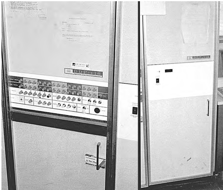
Fig. 6— 6A (left) The DDP-116 Interferometer Control Computer. This photograph was taken in June, 1998, approximately thirty years after the computer began operating the interferometer. The bootstrap loader is keyed in by hand following the recipe written on the inside of the front panel, here shown folded down to reveal the recipe. A supply of panel lights is kept nearby, in the handle of one of the panels. 6B (right). The Rack with the Computer Memory. The black marks at the lower right are said to have resulted from an incident when B. Clark attempted to get the computer's attention.
