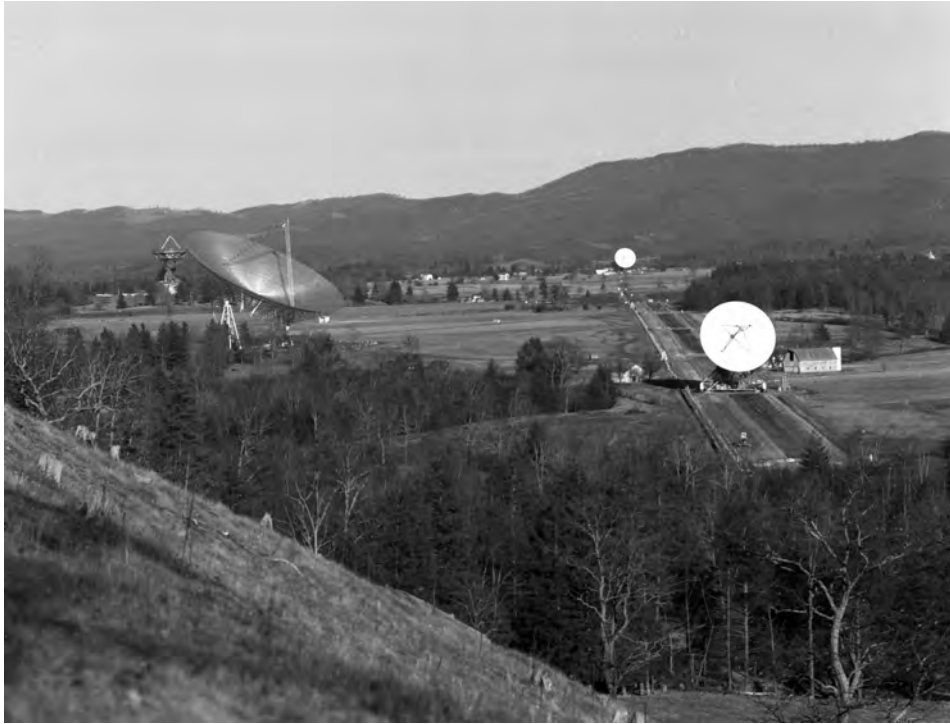
Fig. 3— The two-element interferometer in January 1965. The antenna sits on station 5 (2400 meters), having been moved there for the first time shortly before the photograph was taken. The interferometer backend was in a trailer midway between station 1 (1200 meters) and 85-1; it is, unfortunately, not visible in this photo.
