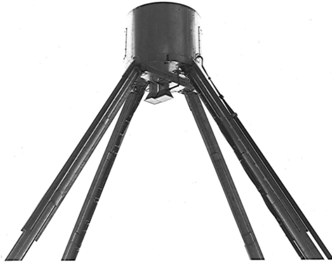
Receiver and dual feed at the focal point of the 85 Foot Tatel Telescope during Project Ozma, 1960.
