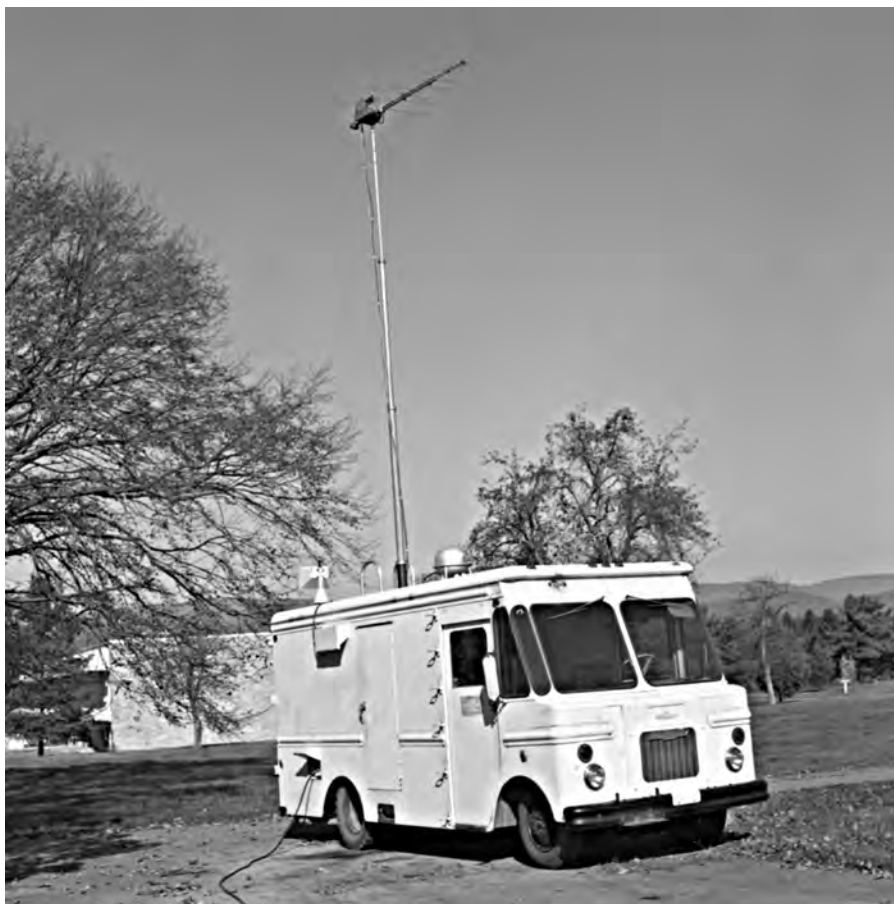
The "Ice Cream Truck," the van used to track down interfering signals, October 1981.
