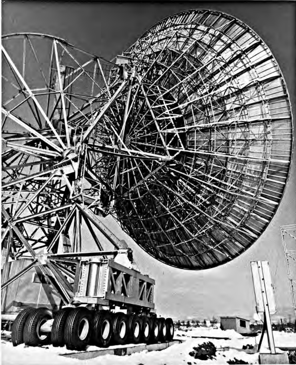
Fig. 1— The second element, 85-2. This telescope was mounted on rubber tires, and was towed along a roadbed in order to move from one antenna pad to another.
