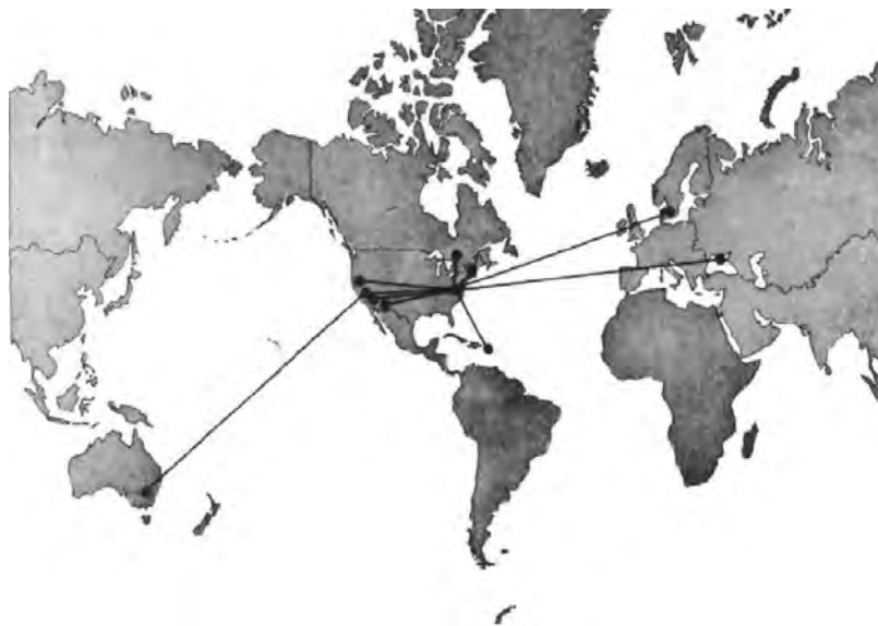
Telescope locations and baselines used in the early VLBI experiments.
