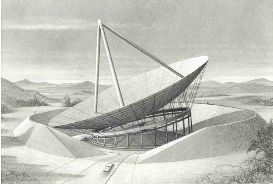
A 300 foot telescope concept with a rotating wedge mount. This design was considered as part of a feasibility study for a 300 foot parabolic antenna with limited steering ability, conducted by the Stanford Research Institute (SRI) for NRAO, July 1960.
