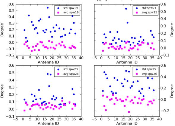
SNR of the phase calibrator {spw19: 63.7, spw21: 101, spw23: 96.6, spw25: 33.1}
