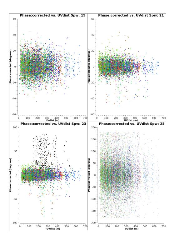
Figure: visibility phase vs uv-distance for phasecal scans (pre-self calibration)
