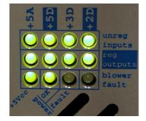
Note that all the LEDs in are bi-color and green indicates 'OK' and red 'fault'. The exception to this are the two bottom right LED's which only light red for 'fault' and are off otherwise.
