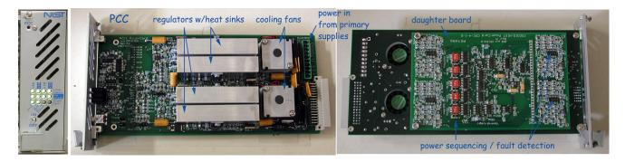
Physically, this card is a double-wide (40 mm) eurocard form-factor (100 x 220 mm) mother/daughter card-arrangement with a 3 x 16 DIN backplane connector for the standard NIST crate backplane.
