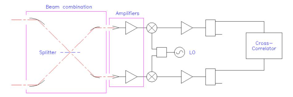
This is the single-dish complement of the two-element spatial interferometer.
