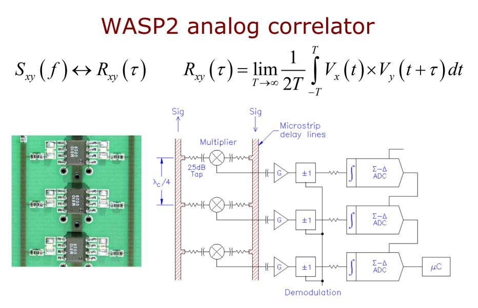
Wideband, simple electronics: low-speed digitization after high frequency delay and multiplication
