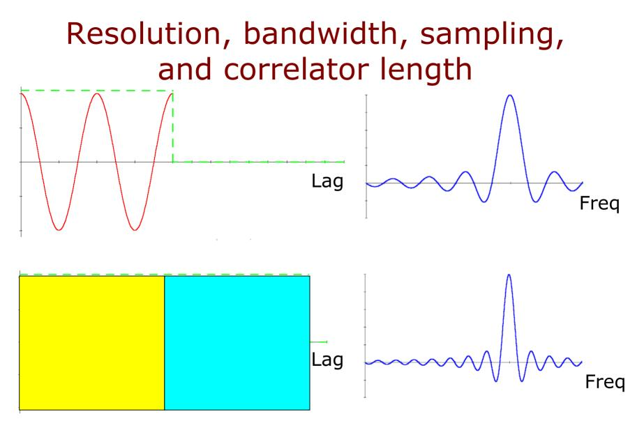
Bandwidth: sampling interval (between lags,  $\lambda_{min}/2$ ) Resolution: spectrometer length ( $\infty$  number of lags)
