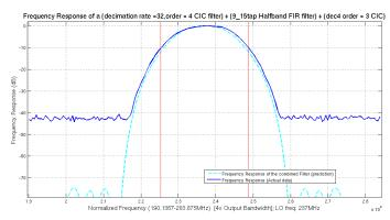
halfband coefficients quantized to FIX16\_14 (as in the model files) final response quantized to 8 bits (as in the hardware)
