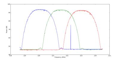
We decdied to use the -6dB response filter as it seems to have better adjacent band rejection and lower sidelobe levels. Below are the theorectical plots:
