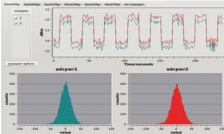
Figure 1: Noise modulation of AP by sig/ref signal as seen in the VEGAS data monitor. ADCpwr1 and ADCpwr2 correspond to the two polarization channels.
