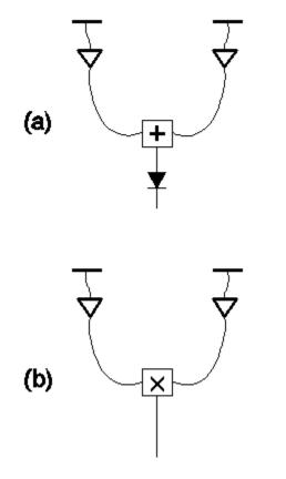
Adding Interferometer or Phased Array
