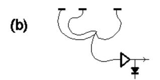
Phased Array. Cables of just the right length, to bring all signals together in phase
