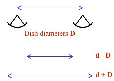
A correlation interferometer of separation d, using dishes of diameter D, includes all baselines from d – D to d + D — Single dish
