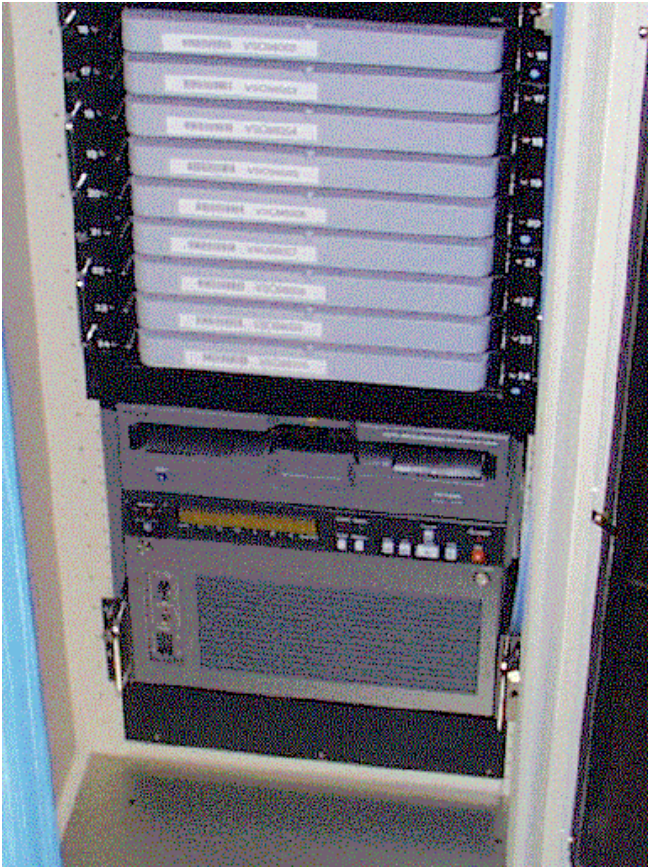
Figure 5: The Data Recorder, DIM-1000M. The recorder is located at the bottom of the rack containing the tape changer.
