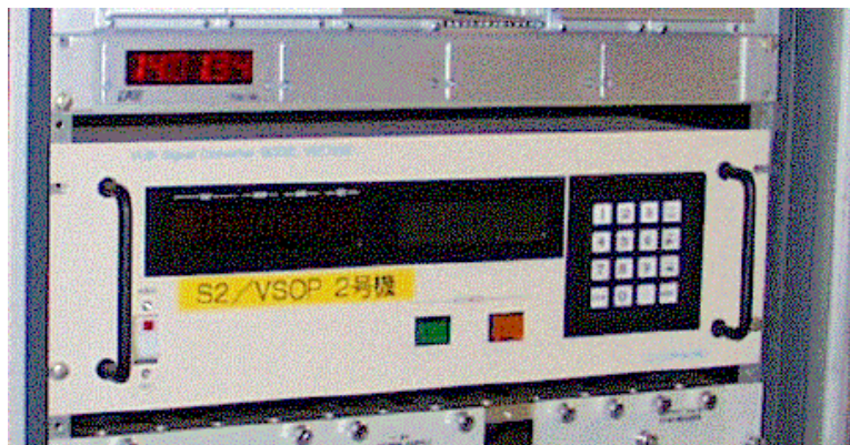
Figure 2: The S2/VSOP VLBI Signal Converter VSC 7220. The upper module is an IRIG clock used to check that the VSOPT recorder is set to the correct time.
