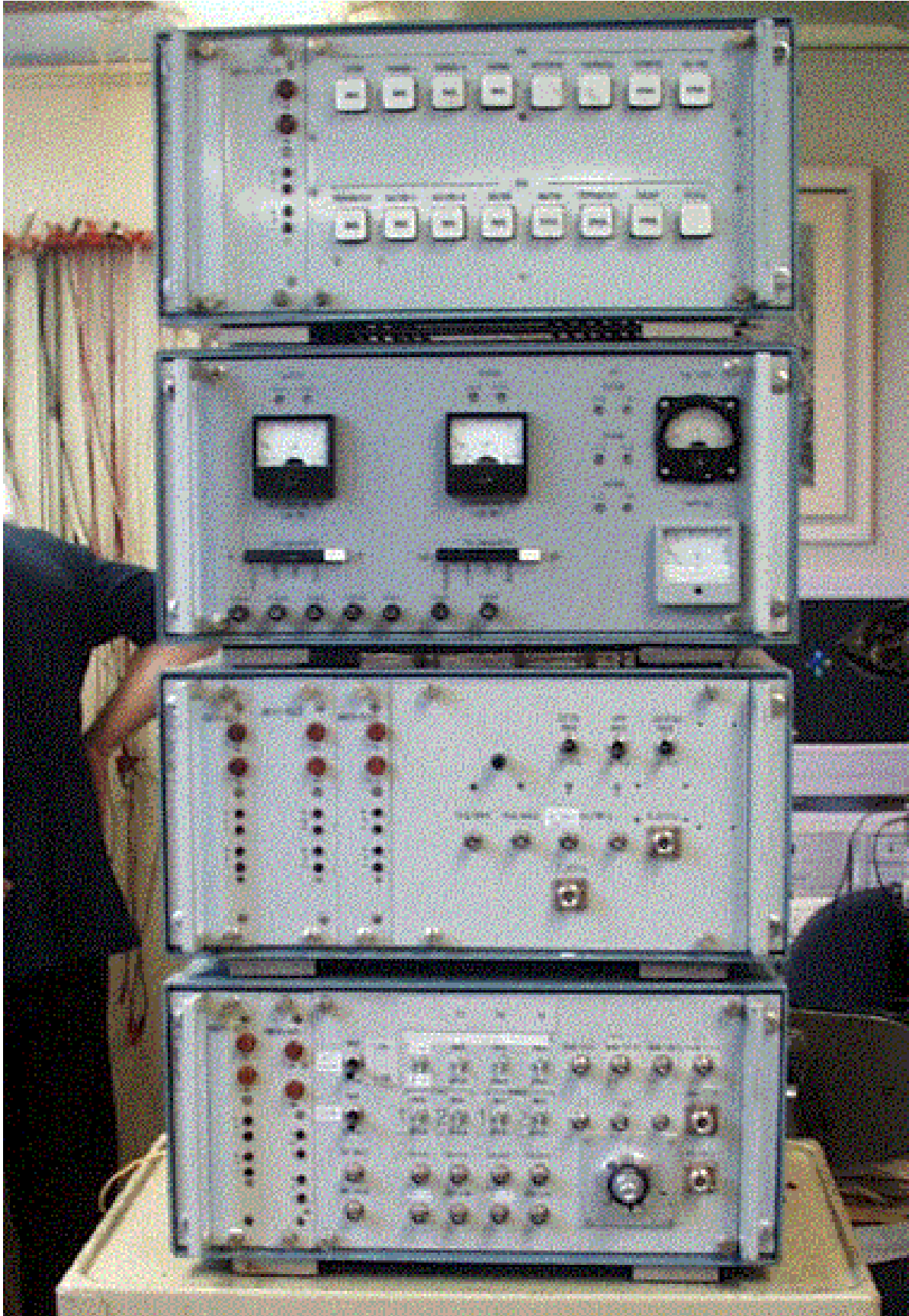
Figure 2: The VIRK test modules seen in the laboratory. The topmost module is the command generator. The next module down is the analog read back module. The bottom two modules are the modulator and the VIRK signal source.
