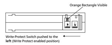
Figure 2-12 Write-Protect Switch on Tape Cartridge
