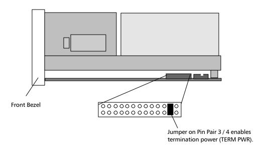
Figure 2–2 Jumper Installed on Pin Pair 3 / 4 Enables Termination Power (TERM PWR)
