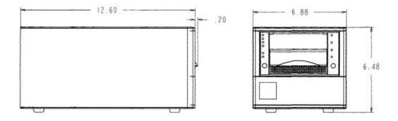
Figure 2-7 Physical Dimensions of DLT 8000 Tabletop System
