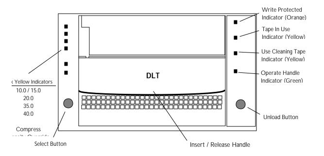
Figure 2–13 Front Panel of Tape System
