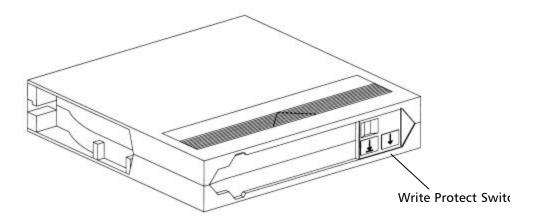
Figure E-5 Location of Write Protect Switch
