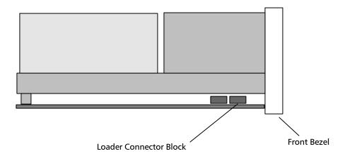
Figure 2–6 Loader Connector Block
