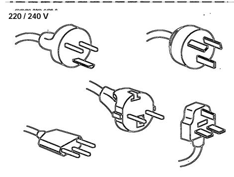
Figure 2-10 AC Power Cord Plug Ends
