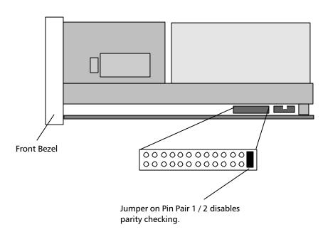
Figure 2-3 Jumper Installed on Pin Pair 1 / 2 Disables Parity Checking
