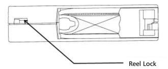
Figure E-1 Location of One of the Two Reel Lock Tabs on the DLTtape
