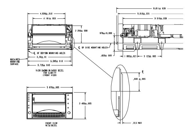
Figure 2-4 Locations and Dimensions for Mounting Holes
