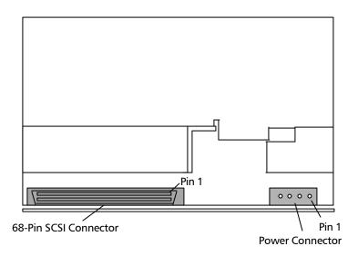
Rear View (Connector End) of Tape System
