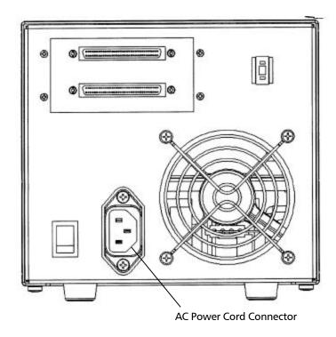
Figure 2–11 Location of AC Power Cord Connector on Rear Panel (Tabletop Version)
