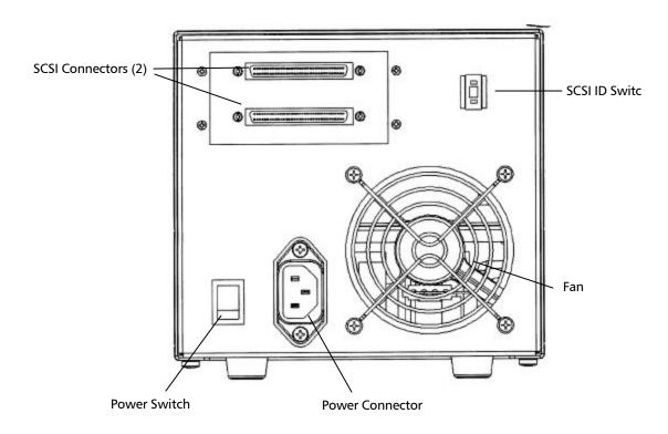
Figure 2-8 DLT 8000 Tabletop Tape System Rear Panel
