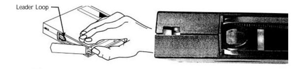
Figure E-3 Opening the Door on a DLTtape Cartridge Showing Tape Leader Loop in its
