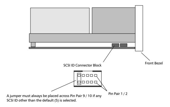
Figure 2–1 Location of SCSI ID Connector Block
