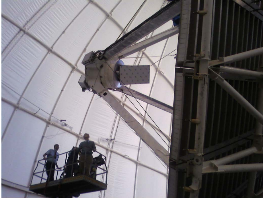
Figure 2 The inclined plane reflector in front of the subreflector redirects the signal received from the radar transmitter directly into the receiver, eliminating the use of the main antenna reflector. In the configuration shown, the signal is being received from the ground.
