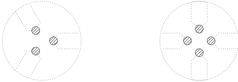
Fig. 8. N -wire model for the low-order modes in ridged waveguides.
