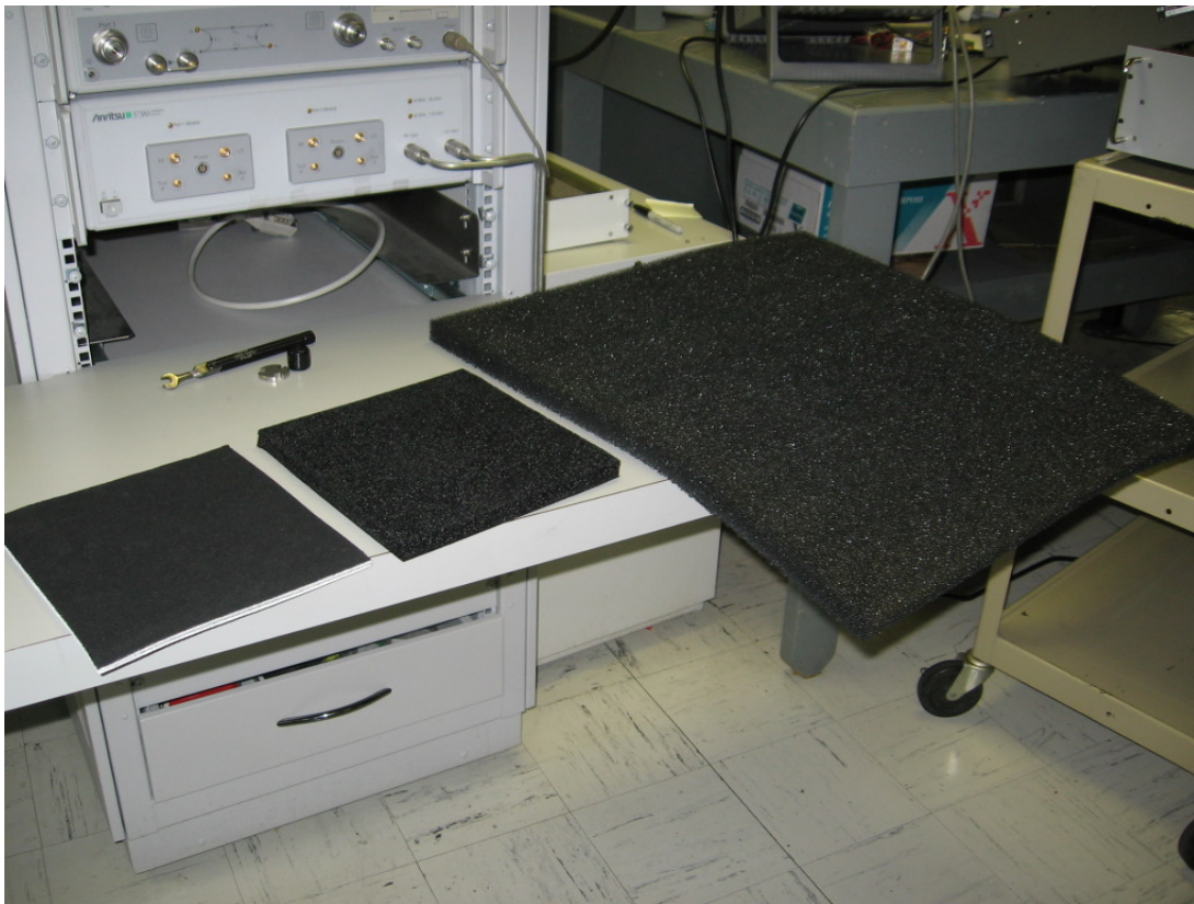
Figure 6: Additional materials tested at W-band. From left, Emerson & Cuming Eccosorb AN-72, Zote Foam LD32CN, Emerson & Cuming Eccosorb HR-25.
