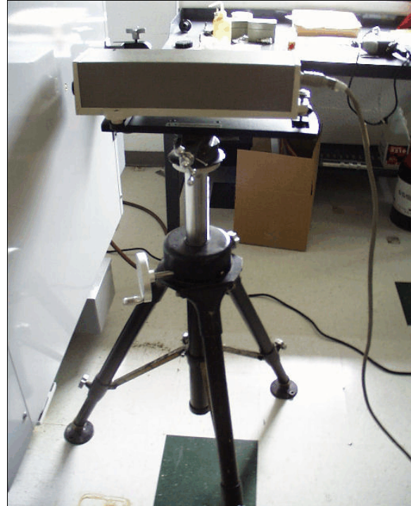
Fig. 8 Laser unit of the HP interferometer as set up for measuring the X-axis. The laser beam enters the mill through a small hole in right cover.
