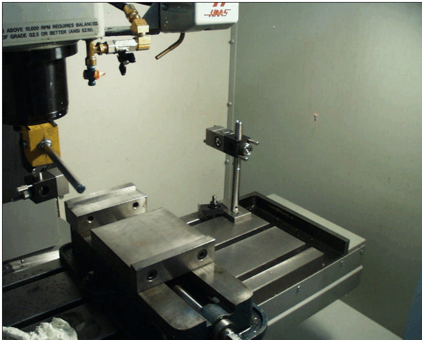
Fig.9 Setup for the X-axis measurements. The beam splitter and retroreflector are at the right on the table of the mill. The retroreflector at the left is attached to the spindle.
