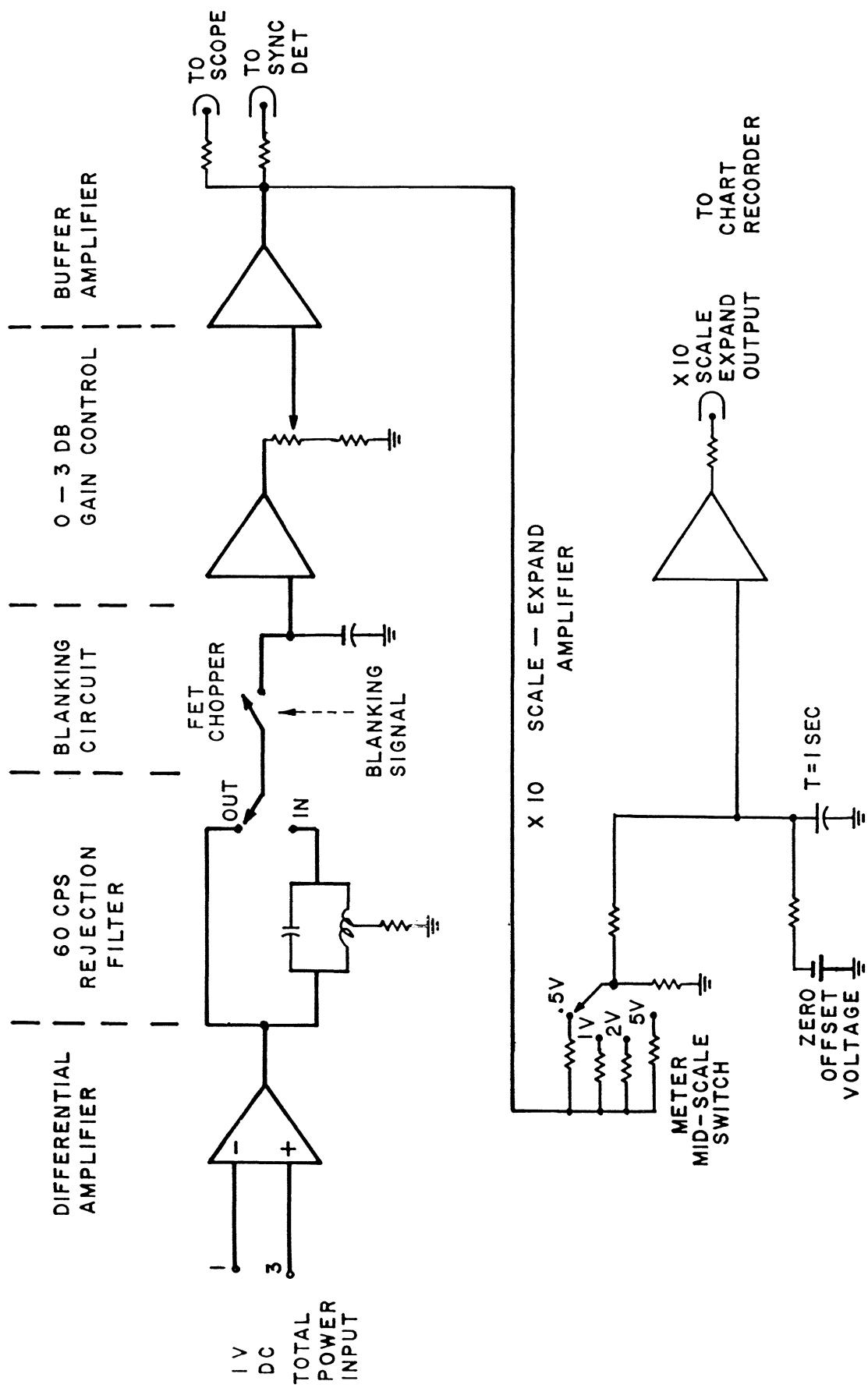
Figure 6 — Total Power Amplifier Block Diagram
