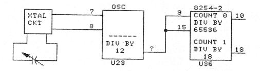
To prevent loading of oscillator I usually monitored pin 9 of  $\rm U_{36}.~$  Two oscillator circuits were used. The first AST used is shown below:
