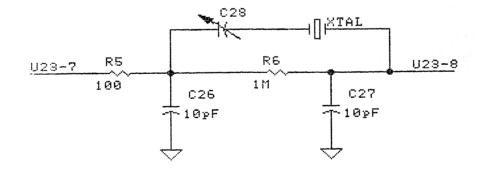
The adjustment range of C28 was not large enough so I had to put 55 pF in parallel with C27. This gave a range of 1.193627 to 1.193139 MHz. When using a counter not locked to maser or Rb 5 MHz, I would read the 5 MHz standard and correct for the offset when setting frequency. I did not record what the AST serial number was.
