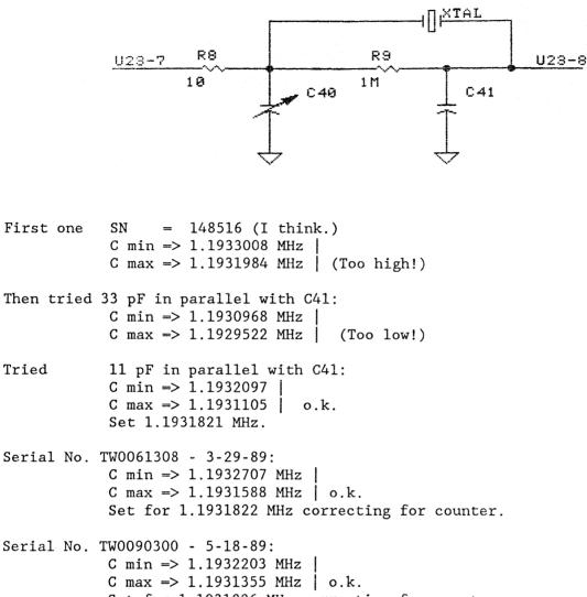
Set for 1.1931826 MHz correcting for counter.
