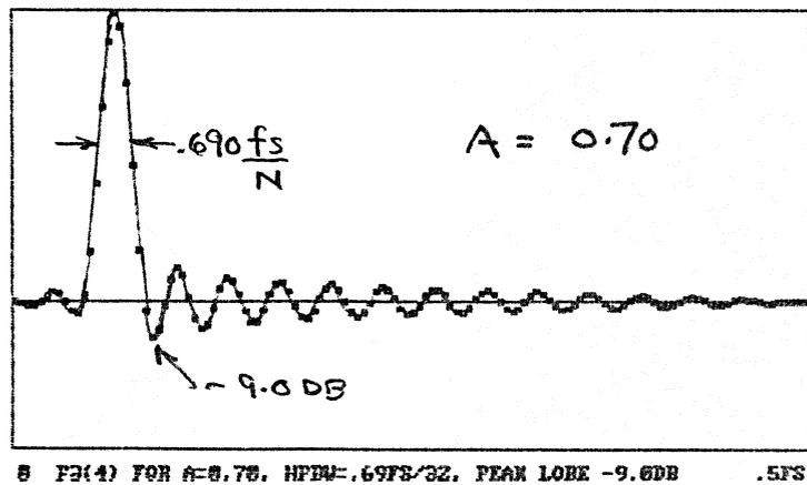
Fig. 4. Response of modified DFT,  $P_3(4)$ , to frequencies from 0 to  $f_s/2$  for weighting factors 0.60, 0.65, and 0.70 which gives increasingly narrow resolution and higher spurious lobe level.
