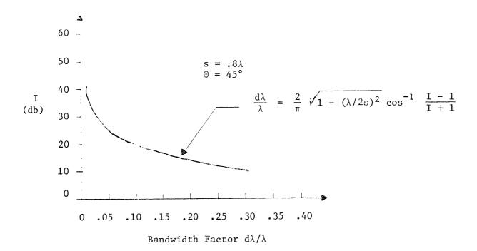
It is seen that the bandwidth factor is about 3% for 30 dB circularity isolation indicating an inherently narrow band characteristic for the polarizer.
