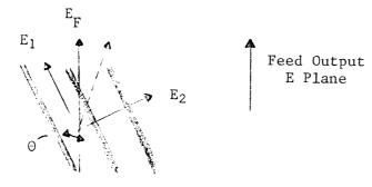
(a)  $\overrightarrow{E}_1$  and  $\overrightarrow{E}_2$  are in time phase for the desired polarization sense. Then:  $E_F = |\overrightarrow{E}_1| \cos \theta + |\overrightarrow{E}_2| \sin \theta$
