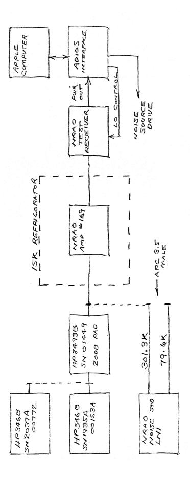
Fig. 1. Test setup for calibration measurements.
