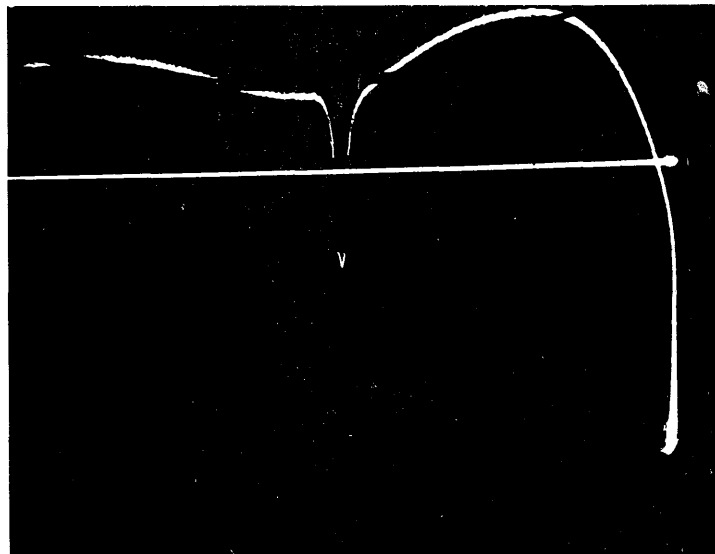
FIGURE 32 GAIN-BANDPASS CHARACTERISTICS OF MPC PARAMETRIC AMPLIFIER FOR 85-2 FRONT-END. SCOPE SENSITIVITY IS 200\mu\text{v/cm} . REFERENCE LINE IS 1 dB POINT. GAIN 15 dB BW 110 MHz RESPONSE FLAT 2725 MHz-2665 MHz = 60 MHz
